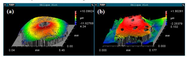
Surface profiles of the 6mm epoxy disk containing the Itokawa particle RA-QD02-0030 (a) and the particle located at the center of the disk (b). The surface profile data were obtained by a ZYGO white light profilometer at the Material Science Center (UW-Madison) before SIMS analyses. In panel a, surface profile data of the central area are lacking, because Au-coating was removed and surface was dim.
