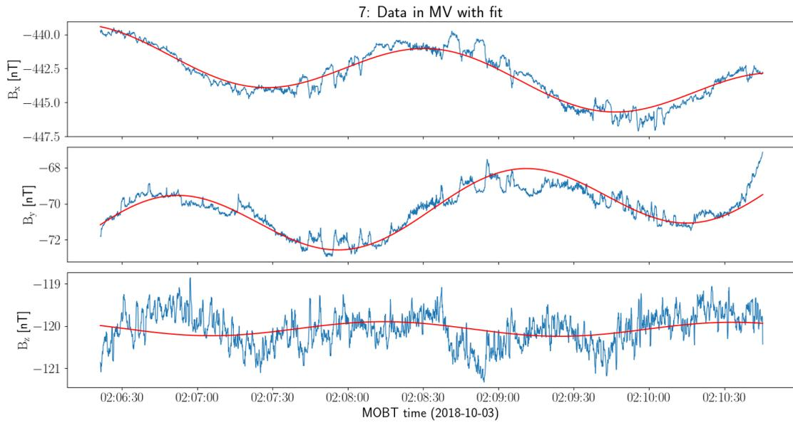
Figure 12: Data in the maximum variance system (blue) with rotational fit (red).
