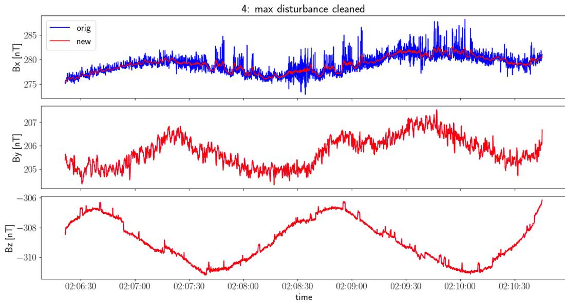
Figure 9: Red curve shows the data cleaned from the high frequency noise (in one axis).
