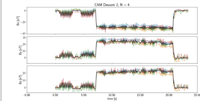
Second sequence of descent signatures of the CAM instrument with slightly worse background conditions.
