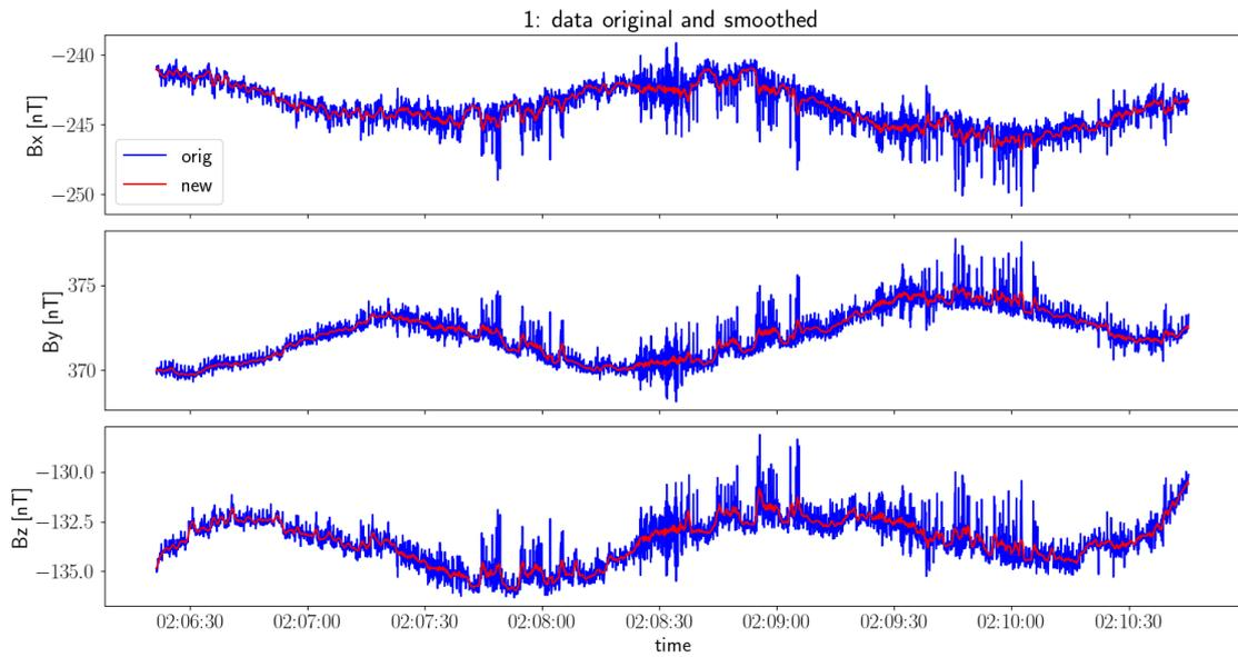
Figure 6: Draft calibrated MAG data (blue) and smoothed data with running average.
