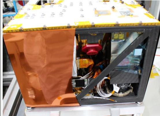
*Figure 2: MasMag as integrated in the MASCOT lander. MasMag sensor is accommodated in the right bottom corner.*
