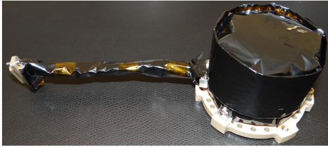
*Figure 1: MasMag sensor wrapped with MLI.*
