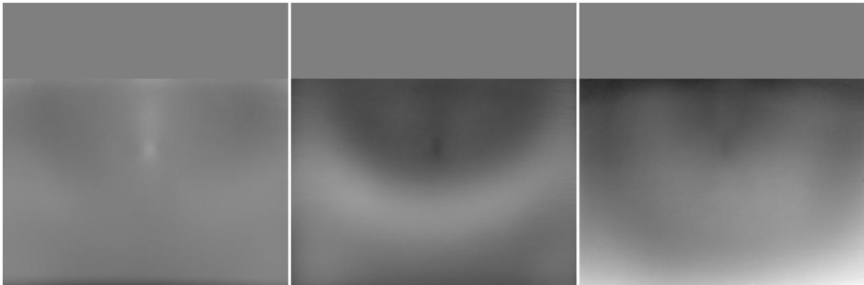
**Figure 5:** LED ratio images. Left: Blue over Green ratio image ( $V_1$ ). Middle: Red over Green ratio image ( $V_3$ ). Right: IR over Green ratio image ( $V_4$ ).  $V_2$  is the unity matrix. The brightness of the ratio images as displayed is such that 0.7 is black and 1.3 is white.
