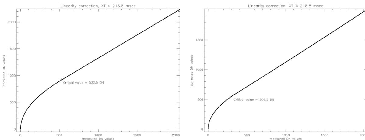
**Figure 3:** Non-linearity curves for short (left) and long (right) exposure regime.
