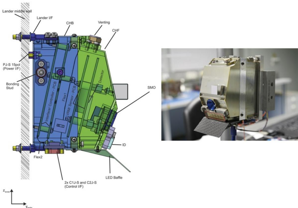
**Figure 2:** Left: MASCOT drawing (CHF = Camera Housing Front, CHB = Camera Housing Back SMO = Surface mode optics, ID=Illumination Device, C1J-S,C2J-S,PJ-S = plug definitions). Right: MasCam flight model
