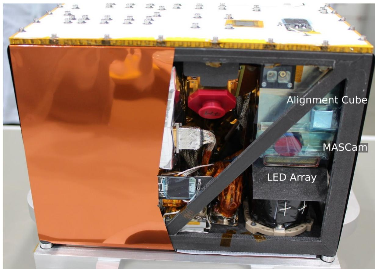
**Figure 1:** Image of the +Y side of Mascot, showing some instruments. The +Z axis of the Mascot coordinate system points down, the +X axis points to the left. The center of the Mascot coordinate system is defined as the center of the bottom plane (not visible). In this image MASCam is visible to the right (towards the -X direction of Mascot).
