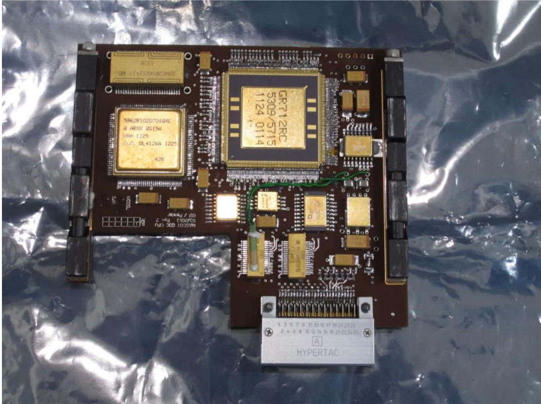
Figure C3 Photo of the CPU (main) board, top side (B. Cozzoni, pers. comm.)
