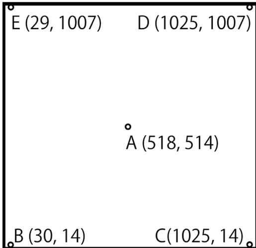
**Fig. 13** Positions where PSFs were measured
