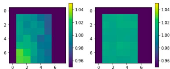
**Fig. 3 Ratio between two aligned images binned in 128 x 128 pixels. Old flat-fields (left) and new flat-fields (right) were applied. One which new flat-fields are applied show better flatness.**
