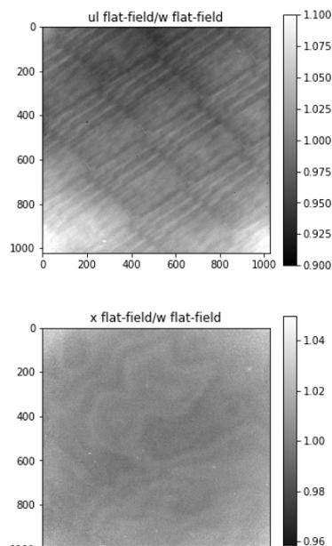
**Fig. 1 Old flat-field patterns for ul-band (top) and x-band (bottom).**
