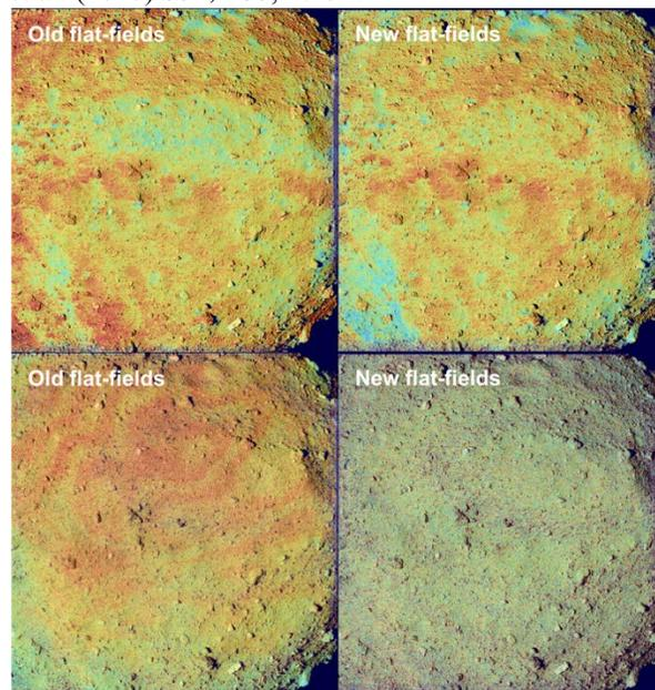
**Fig. 4 Spectral feature maps using old and new flat-fields: spectral slope (top) and 0.7- $\mu\text{m}$  band absorption (bottom).**
