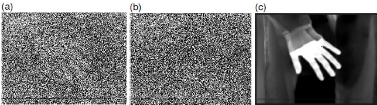
Figure 4 Examples of images obtained by LIR. (a) A raw target image, (b) a raw shutter image, and (c) the resultant image produced by subtracting the shutter image from the target image (Fukuhara+2011).
